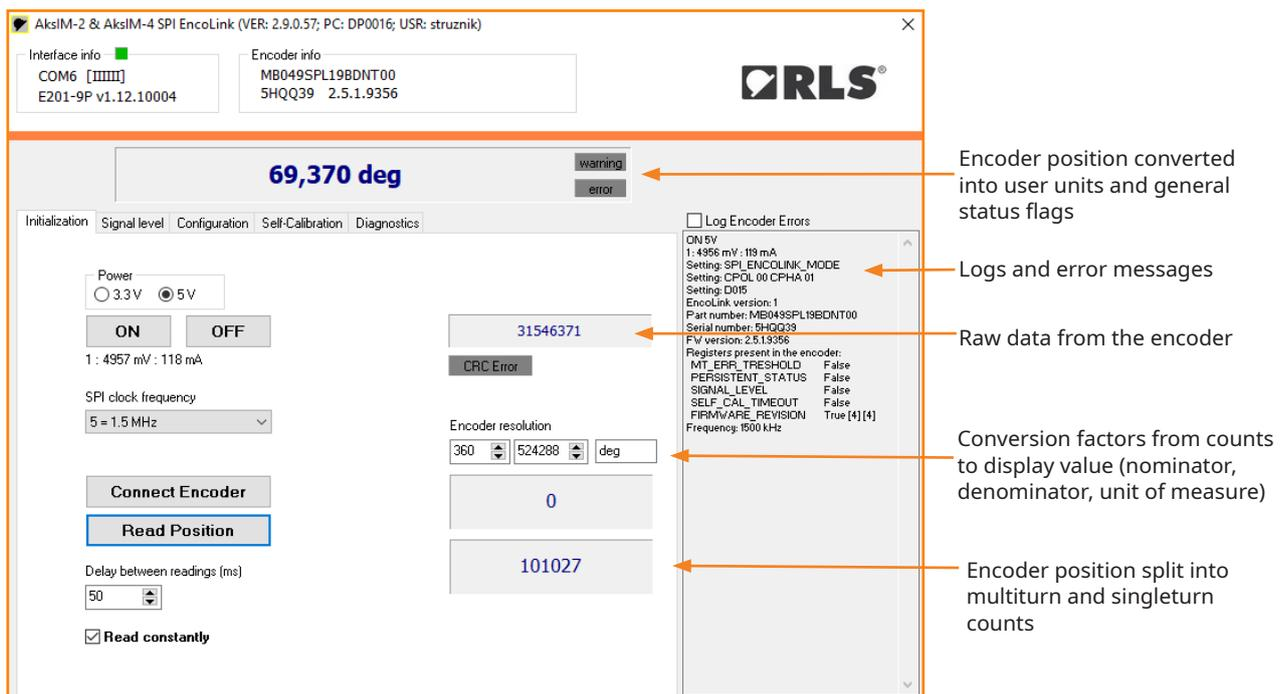
3. Air gap and temperature of the encoder can be logged in the section "Signal level" (check the boxes first). Errors can be logged for further analysis.
