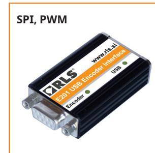
For use with absolute encoders with SPI or PWM communication interface.
